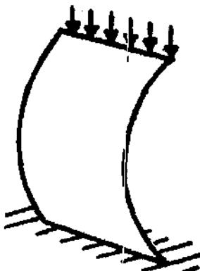
2. The thin skin of an aircraft does not have sufficient bending stiffness to keep its shape under loads. For that reason it is stiffened with so called stiffeners. Which two statements concerning stiffeners are false?
