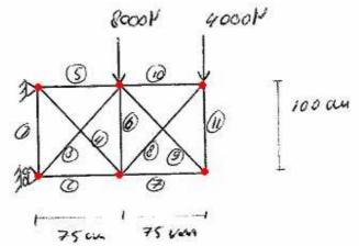
Okay, just like before, Abdalla started with the determination of the statically indeterminacy.
