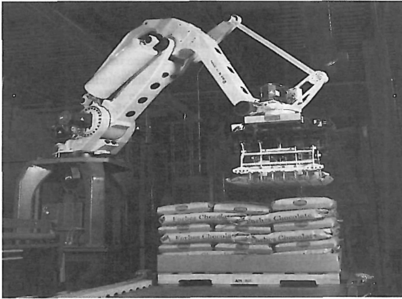
FIGURE 6.11 The FANUC M-410iB™ has 4 axes of motion. It is seen here moving and stacking sacks of chocolate
