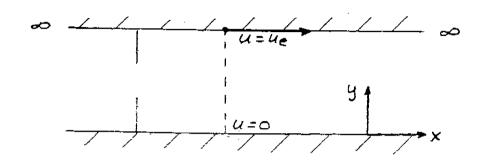
(a) Since the plates are infinite in length, u = u(y) only. Also, v = 0, i.e., the flow is in the x-direction only. The governing equation is Eq. (15.18a), which reduces to the following u = u(y), v = 0 and p = const.
