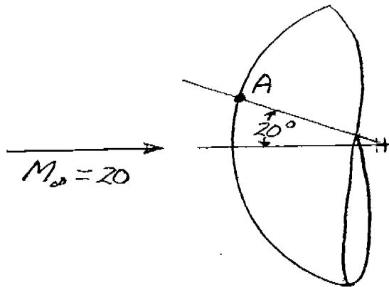
(a) Use Eq. (14.7) to estimate the pressure at point A. We first need to obtain  $C_{p,\max}$ , which is a function of  $p_{0,2}/p_\infty$ . From Appendix B for  $M_\infty = 20$ ,  $p_{0,2}/p_\infty = 0.5155 \times 10^3$ . Hence,
