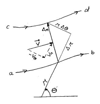
Mass flow between streamlines =  $\Delta \bar{\psi}$
