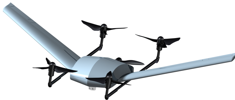
Figure 15.1: Overall configuration of the silent delivery drone
